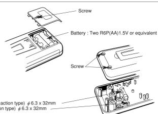
Fuse: F 600V/10A (Fast action type)  $\phi$  6.3 x 32mm F 600V/800mA (Fast action type)  $\phi$  6.3 x 32mm —
